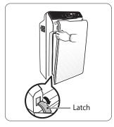
② Remove the filters from the unit, they are protected inside a plastic wrap
